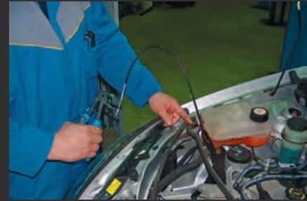
Automatic pliers for spring clamps can be used for clamps that are mounted in the most inaccessible places.
