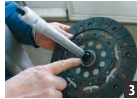
Insert the centering tool into the disc.
