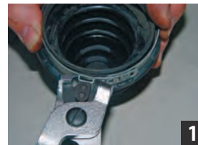
To mount cuffs, Oetiker coupling clamps are used that can only be mounted with special pliers.
