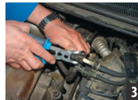
With pliers for clamps for fuel, release the clamp so that the pipe can be removed.
