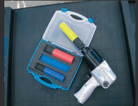
Variously coloured impact sockets with plastic protection for pneumatic hammer
