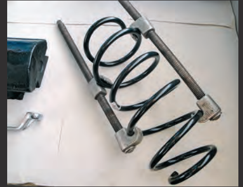
The older version of a simple tool for removing shock absorbers, which is not reliable enough.
