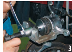
By rotating the handle or by using a socket wrench, push the brake piston into the starting position.
