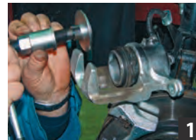
Mount the body of the tools with the suitable thread for compressing the pistons on the caliper.
