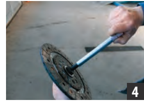
Fasten the tensioning screw so that the tool completely fits the disc.
