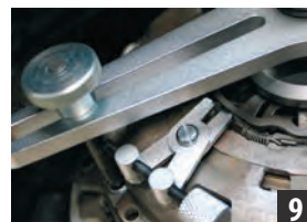
Insert the tool for the tensioning screw.
