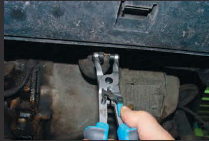
The pliers have a stop that holds the spring open so that the clamp can be removed easily.
