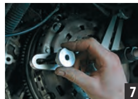
Fasten the nuts onto the tensioner.
