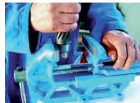
The quick travel guide is raised and the jaw is moved without rotating the spindle.
