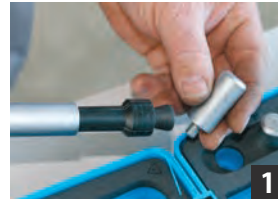
Choose a socket of a suitable size.
