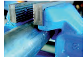
The lower end of the jaw is designed for clamping of tubes.
