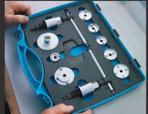
A suitable adapter that accurately fits the size of the brake piston must be selected.
