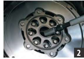
The socket size should suit the flywheel.
