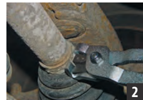
The pliers deform the ear of the clamp so that it can no longer be opened.
