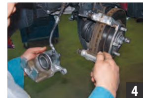
Replace the brake pads or even the brake disc.
