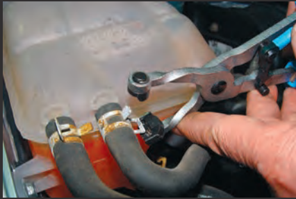
Spring clamps have a relatively strong spring that can only be opened in an easy way using special pliers.
