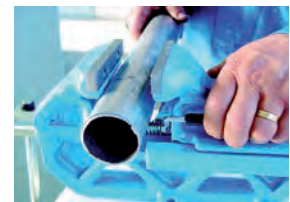
The vice with quick travel is also equipped with jaws for gripping tubes.
