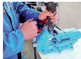
For a firm grip, the spindle handle must be turned only by a half of the circle.
