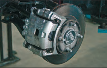
When replacing the brake pads, the brake calliper must first be unscrewed and removed.
