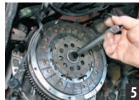
Insert the disc with the tool into the spindle.
