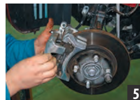
Remove the disc spreader and mount the brake caliper on the mounting boss.
